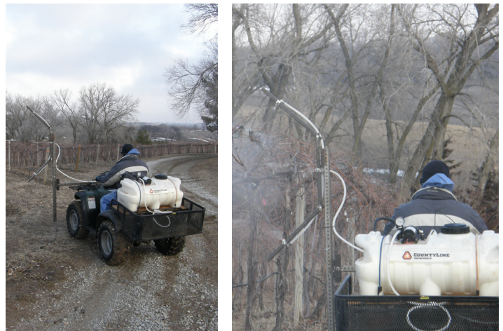
Figure 1. ATV sprayer modified to spray Amigo Oil and NAA to unpruned vines. An adjustable lateral and vertical support arm was attached to the front of the ATV and three flat fan spray nozzles were attached to adjustable arms that surround the cordon. The small droplets easily penetrate into the cordon area and cover all buds. The sprayer was also equipped with a tank agitator, which kept the oil and NAA in suspension, allowing more even coverage of the material.
