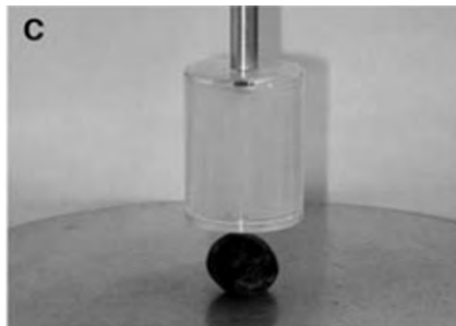
Figure 4. Example of texture analysis for measuring fruit firmness using c) a compression test and f) a puncture test (Rolle et al., 2012).
