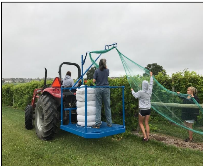
Figure 1. Applying nets in the vineyard at WMARS. The new system consisting of a hand powered platform with a net applicator mounted on a tractor. The system can be operated by 3 people, a driving and 2 others positioning the nets on both sides of the row.
