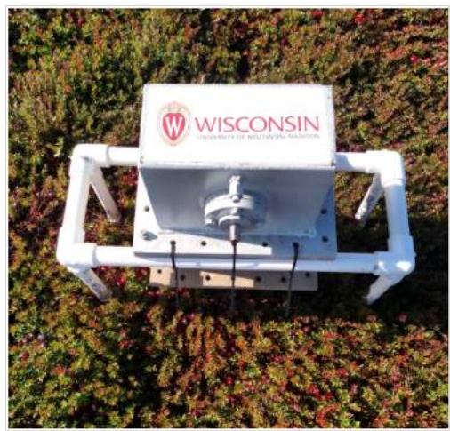
Fig. 2. A microwave waveguide suspended above the canopy surface in a cranberry bed in central Wisconsin.
