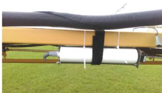
Figure A. SPLAT extruders mounted onto a boom sprayer.
