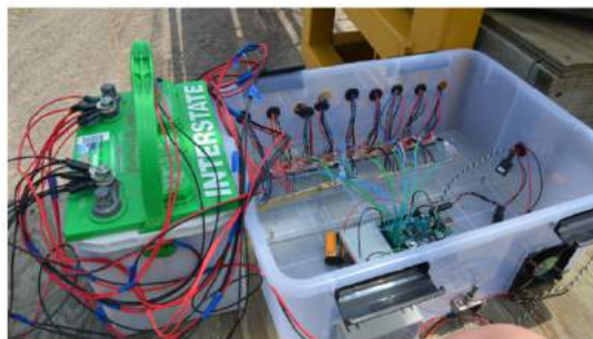
Figure C. Electronic components programmed to dispense SPLAT at ideal dollop rate and 12 volt battery to power system.
