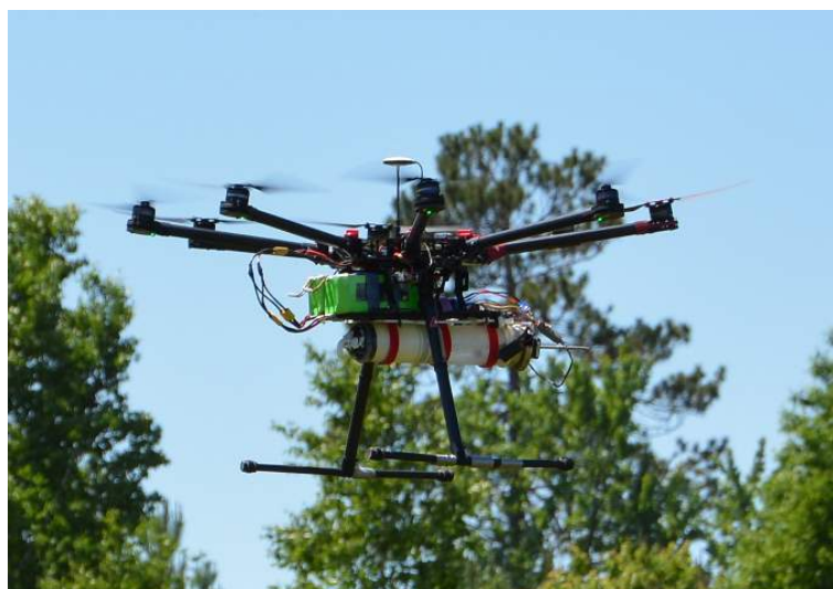
Figure 2. Retrofitted drone, applying MD product to commercial cranberries.
