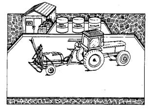
concrete pad. Make sure that the sump drain valve (if installed) is locked in the closed position. Pump any leftover field-strength chemical and rinse water from the sprayer drain valve into a marked rinsate tank.
